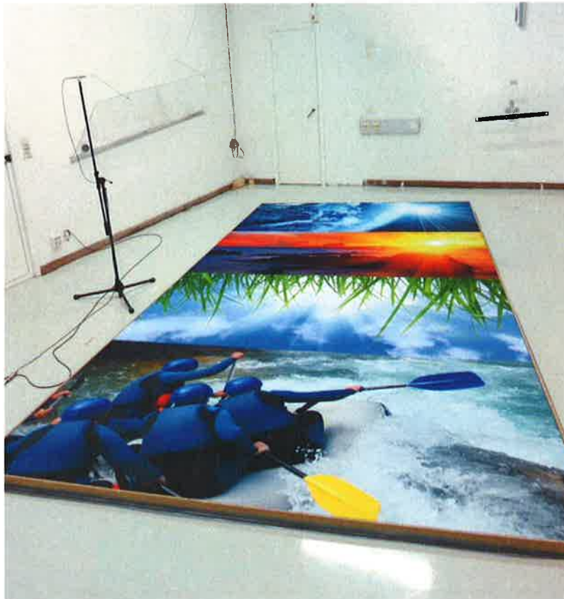
Specimen in reverberation room.
